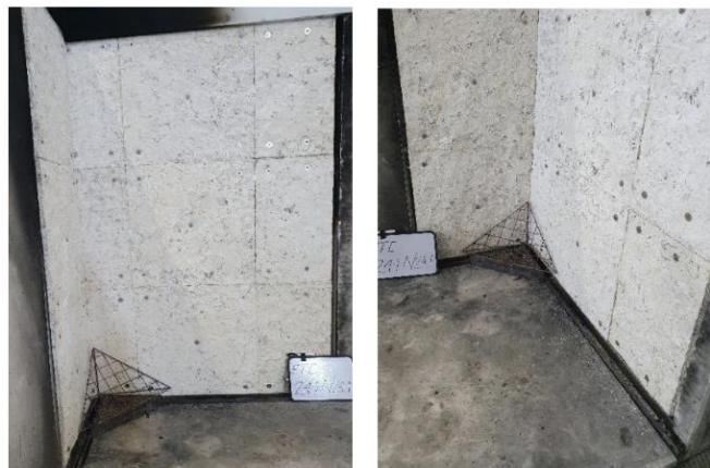
Fig 10. LD panels with “Gyptec BA F 13” gypsum boards .
